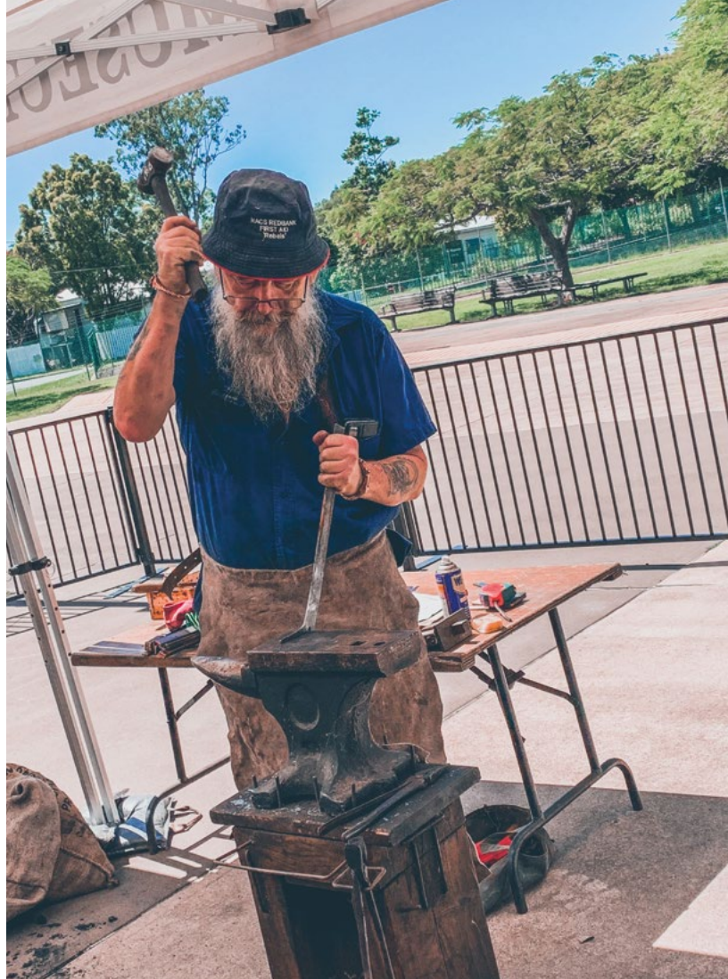
LEFT: Instructor Rob using the anvil to start shaping a french-style carving fork.
